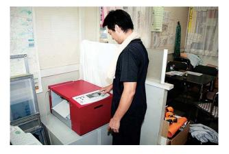
the strengths of of the ne GOCCOPRO 100 is we are able to screen-print directly from PC data. In the past, we have printed a hard copy from PC data and we have made a positive from a hard copy using a scanner. It reads unnecessary impurities of paper and smudge of scanner, and then this has often caused pin holes. This was our big headache, but the GOCCOPRO 100 that directly reads and writes the data has got rid of our headache.
