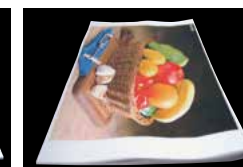
Deformations such as waves and curls easily arise with water-based ink.
