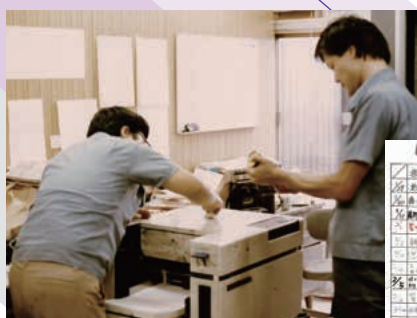
“One million page test” that was carried out in shifts by groups of two people and a progress chart on which each supervisor recorded test results
