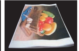
Deformations such as waves and curls easily arise with water-based ink.
