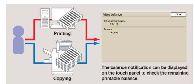
**Notifying users' printing status:** By displaying pop-up screens on PC or sending e-mails, the remaining printing credits and usage conditions will be notified. In addition, various detailed information including the number of print jobs and number of printing sheets can be also checked.
